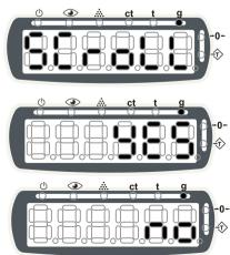
press the MODE button, and user can choose whether the scrolling function is required or not. If the price scrolling function is required user should select "Yes", and if it is not required then the user should select "No". Press the ZERO button, to exit this setting. Now the scale will scroll the rate entered in the price entering function, that is when the scale is switched on and idle, the display will start scrolling "today's rate 10 gm 5500"
