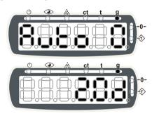
the value using the MODE (M) button. 3.0d means 3 divisions Default setting of Auto-Zero mode is 3d.
